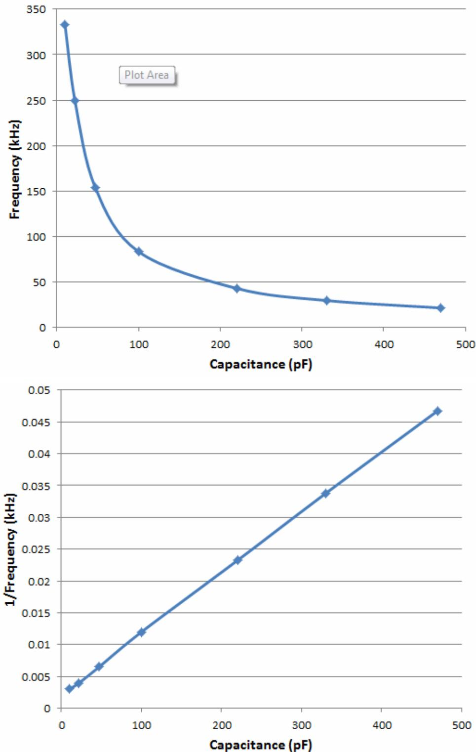
Figure 2: Plots of Frequency & 1/Frequency vs Capacitance
