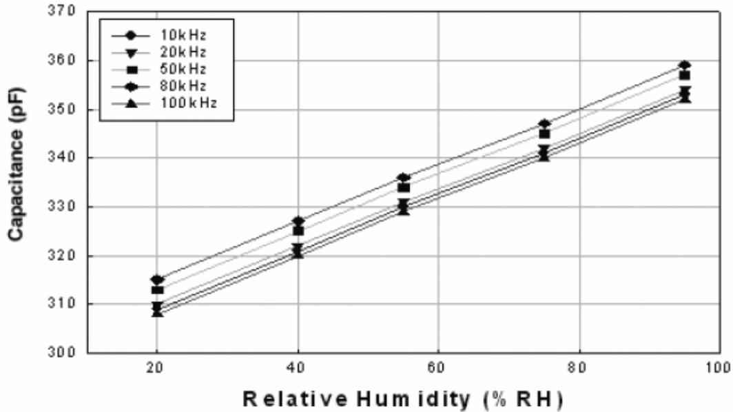
**Figure 6: Plot of Capacitance vs Humidity for HCH-1000**
