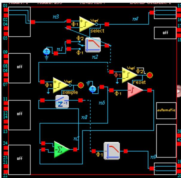
**Figure 3: Oscillator + Frequency to Voltage Converter**
