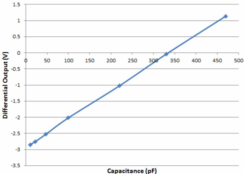
**Figure 4: Plot of Output Voltage vs Capacitance**
