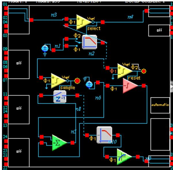
**Figure 5: Oscillator + F2V Converter + Linearization**
