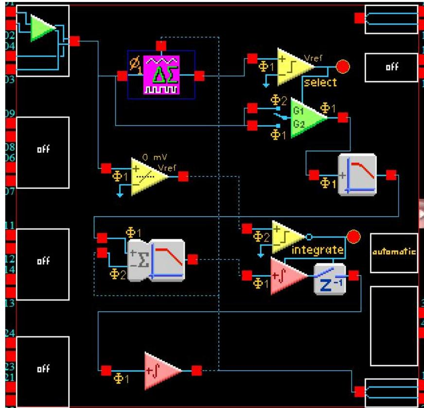
Figure 6: RMS to DC converter
