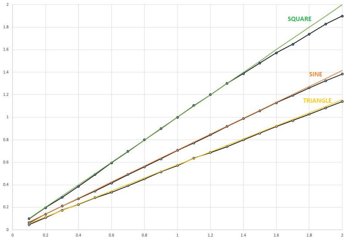
Figure 7: RMS output vs input, measured vs theoretical
