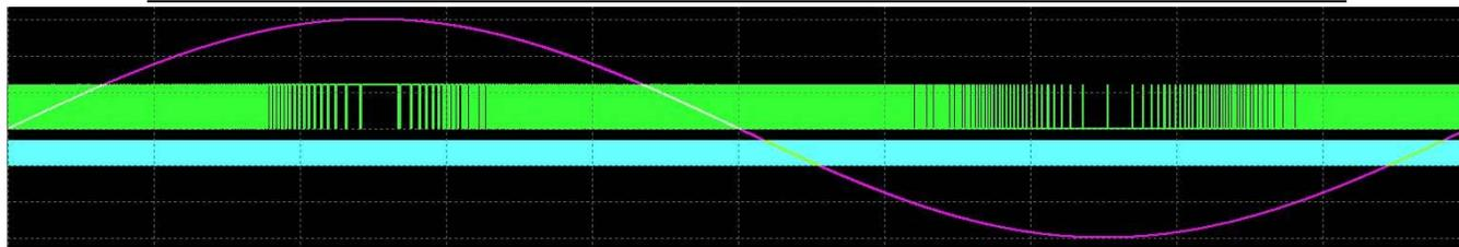
Figure 3: DeltaSigma PDM O/P for 1KHz sinewave, 4MHz clock
