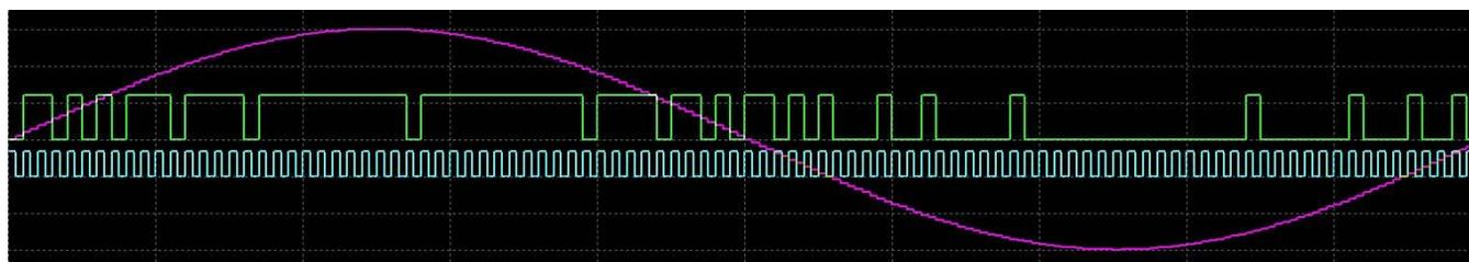
Figure 2: DeltaSigma PDM O/P for 1KHz sinewave, 100kHz clock
