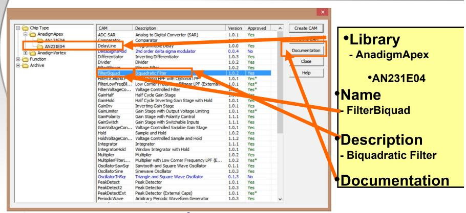
In AnadigmDesigner®2, CAMs may contain multiple circuit configurations. Select the basic function. The details will be set during CAM configuration.
