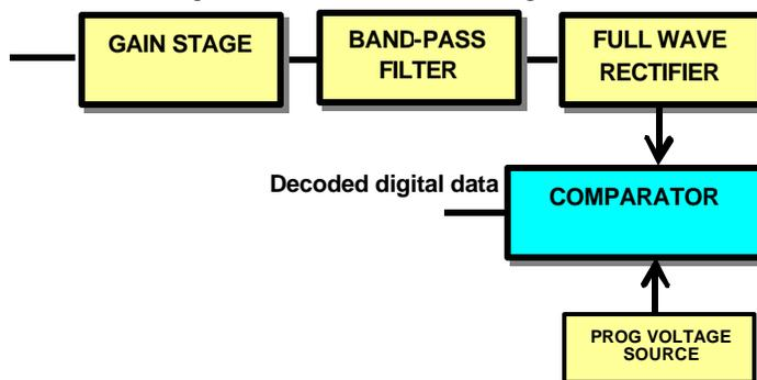
Following Figure 2 from left to right the signal processing chain begins with a simple gain stage. This is used to provide maximum voltage swing within the FPAA.
