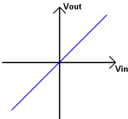
Figure 1: Transfer Function of an Amplifier
