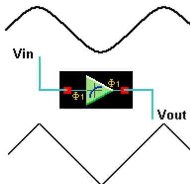
Figure 3: Effect of “Inverse Sine” Transfer Function
