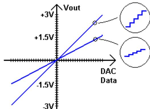
Figure 7: Quantization of the Output Voltage
