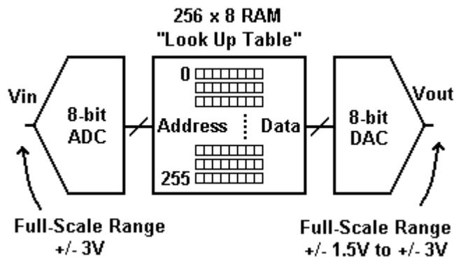
Figure 4: Block Diagram of TransferFunction CAM
