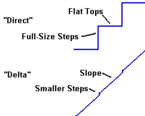
Figure 10: “Direct” Versus “Delta” Quantization
