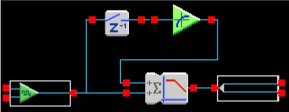
Figure 11: Example “linearization” circuit
