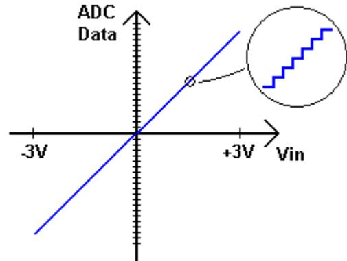
Figure 6: Quantization of the Input Voltage
